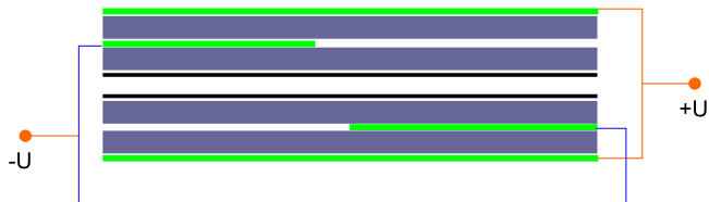
FIG. 7. (Color online) Proposed device setup to measure the 1D ZLM in bilayer graphene. The black solid lines represent the bilayer graphene and green lines represent the gate electrodes. The dielectric barrier materials are depicted in dark blue. In this setup, only the two local gate electrodes need to be aligned.
